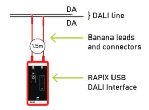
Functions which require a connection to a DALI line only (PC connection not required)
